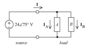
$$\mathbf{I}_{A} = \left(\frac{2(14.12 + j8.47)}{24\angle75^{\circ}}\right)^{*} = 1.37\angle44^{\circ} \text{ A}$$
